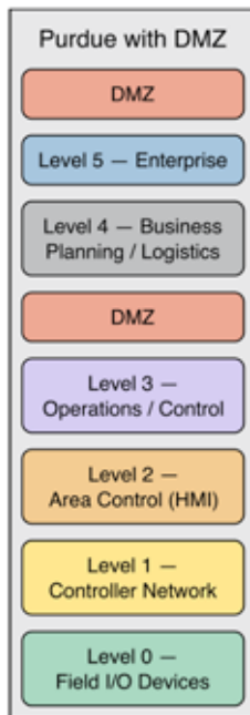
Fig. 2 - “Reference architecture for segmented IT/OT with an industrial DMZ and jump host.” Adapted from NIST SP 800-82 Rev. 3, Sec. 5 (public domain).
