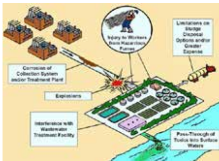
Impact of untreated industrial WW discharges.
