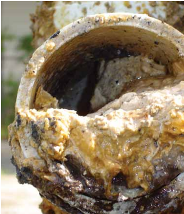
Sewer pipe clogged by Fat, Oil and Grease (FOG) buildup
